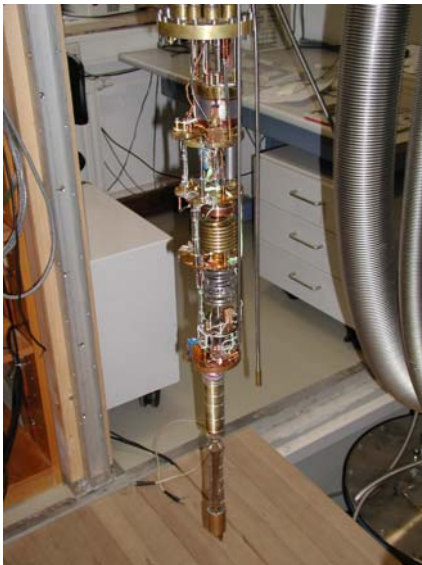
The "cold finger" which holds the QC chip (the cold finger is submerged in the white barrel that appears in the photo above)
