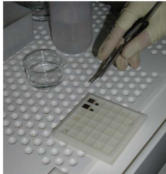
QC chips, which are aluminum and niobium on sapphire – they are mounted at the bottom of the cold finger
