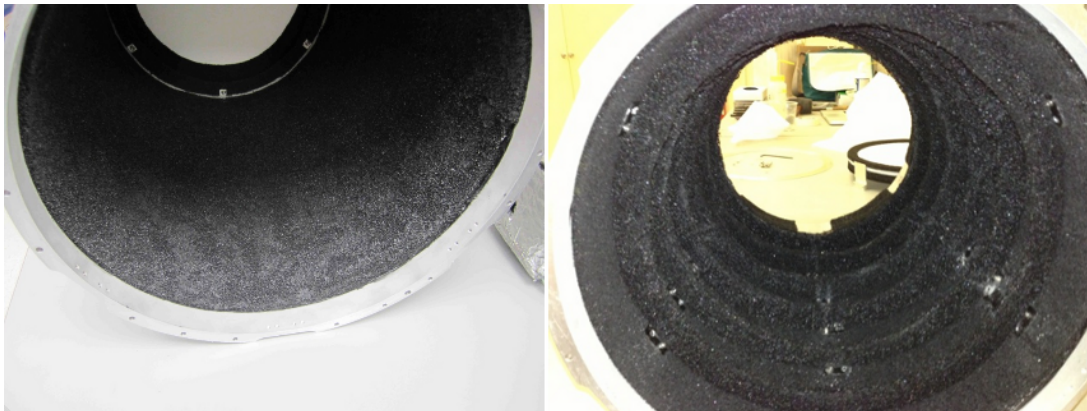
Figure 5. In order to reduce detector loading from the warm forebaffles, we added baffles inside the cold telescope tubes of the Keck Array for the 2014 season. Left: A Keck Array telescope tube as configured for the 2011–2013 observing seasons. In this configuration, shallow-incidence reflections off the telescope walls allowed a significant amount of forebaffle emission to reach the detectors. Right: A Keck Array telescope tube with baffles added as configured for the 2014 season. We oriented the baffles so that any such shallow-incidence rays would be at near-normal incidence on the baffles and therefore absorbed efficiently on the cold telescope walls.
