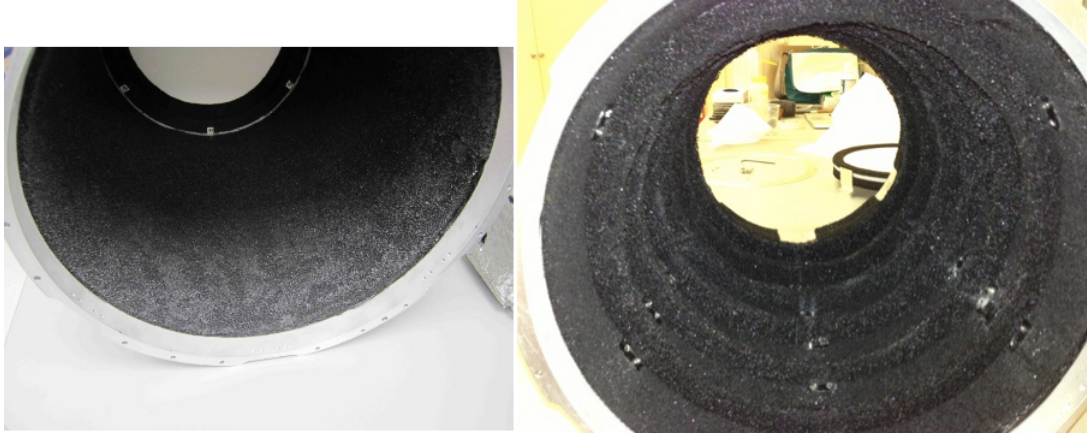
Figure 5. In order to reduce detector loading from the warm forebaffles, we added baffles inside the cold telescope tubes of Keck Array for the 2014 season. Left: Shallow-incidence reflections off the telescope walls created an unintended coupling between the forebaffles and the detectors. Right: The baffles are oriented so that any such shallow-incidence rays will be at near-normal incidence on the baffles and therefore absorbed efficiently.
