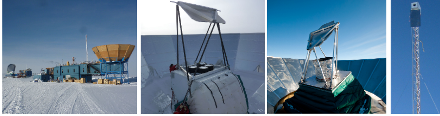
Figure 1. To make far-field beam maps we put microwave sources on masts and use flat mirrors to redirect the radiation into our telescopes. Left: The Dark Sector Laboratory (background) and Martin A. Pomerantz Observatory (foreground), housing BICEP2 and Keck Array , respectively. Each building has a mast for far-field beam mapping, and the distance from source to telescope is 211 m. Center Left: The flat mirror installed above Keck Array . Center Right: The flat mirror installed above BICEP2. Right: We enclose the microwave source on top of the mast in an absorptive box so that only radiation emitted from the intended aperture reaches the telescope.
